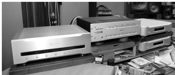
Rubidium master clock generator G-0Rb (left). A set of D/A mono-block converters D-01VU (right).
