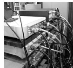
Rubidium master clock generator G-0Rb (left). A set of D/A mono-block converters D-01VU (right).
